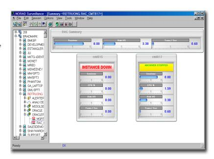
At one glance you see the overall status of the RAC. Nodes that are up are displayed in green. Nodes that are down are red. The RAC status window also shows user counts, CPU usage, I/O, transaction throughput and the general status for each node and the entire RAC.
